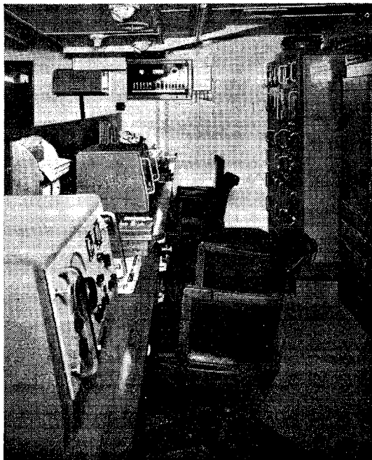
Two of the receiving positions in the Caronia . The single sideband receiver is seen in the right rear alongside the telephone terminal equipment
